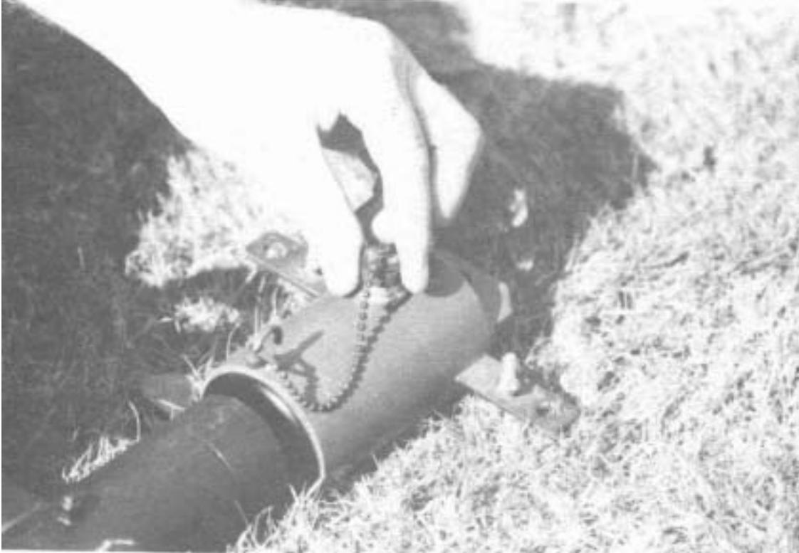
Ensure that the coaxial connector protective dust cap is in place when the antenna is not in use.
