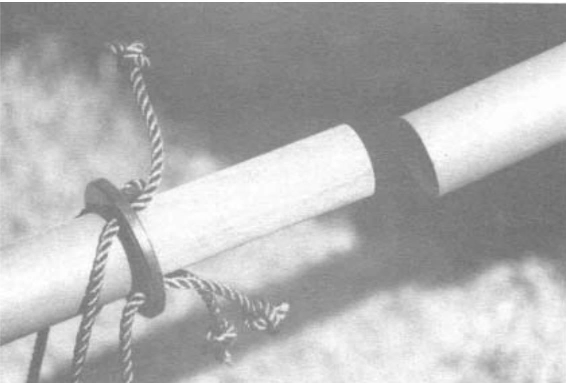
Guy ring on the spigot shoulder, with the reset mast section ready to locate. Note that the knots are pulled clear of the shoulder, so that the locating section sits squarely on the guy ring.
