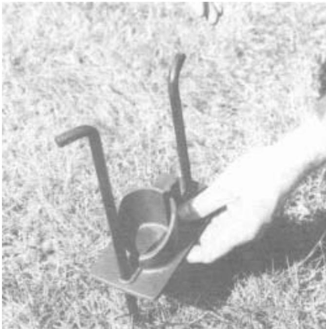
Pinning the mast base to the ground.
