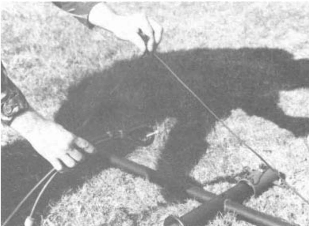
Ensure that coaxial cable is passed under the crossarm catenary.
